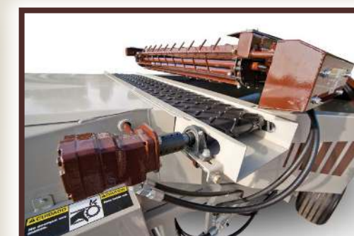
Stick discharge belts are standard on all De-Sticker carts.
