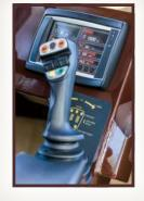
Multi-function joystick and large touchscreen display for comprehensive diagnostics, control settings and load mode
