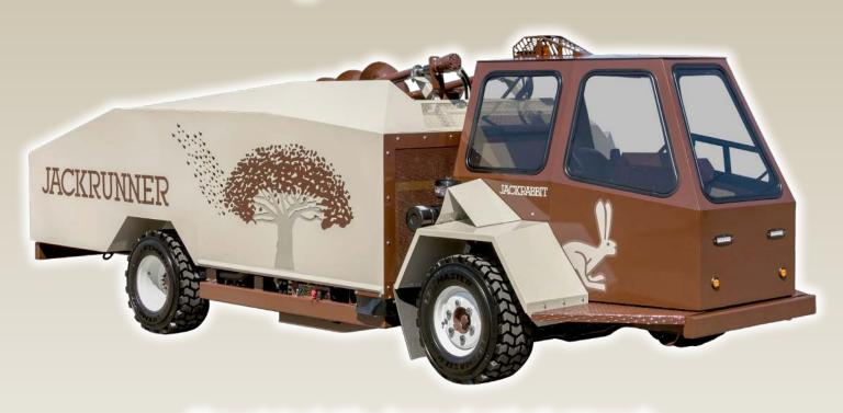
The original side-dump shuttle that travels up to 35 mph in both directions
