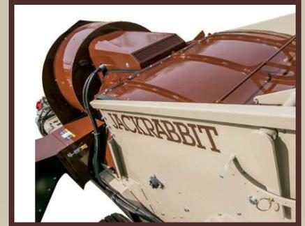
Adjustable damper to fine tune airflow
