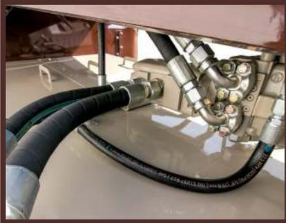
Hydrostatic pump for variable fan speed
