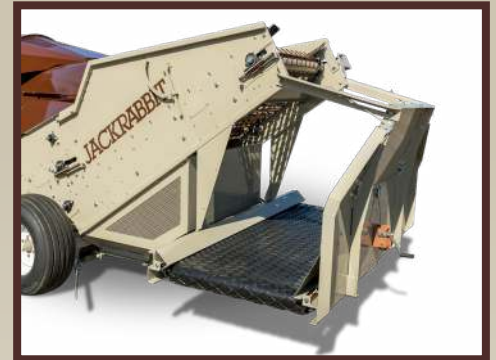
Large collection bin with bi-directional conveyor belt
