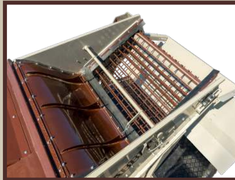
Heavy duty stick chain to remove unwanted sticks and debris
