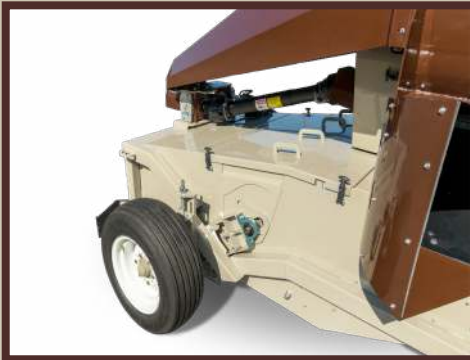
Removable pickup head cartridge for ease of service and repair
