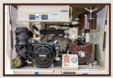
Carbon monoxide rich exhaust is cooled and passed through a vacuum pump for maximum volume and velocity.
